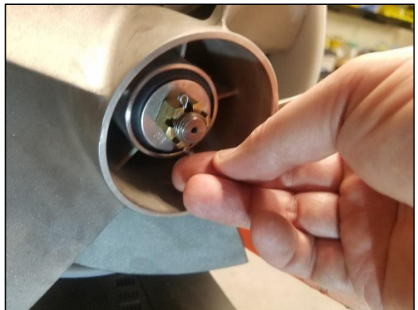
Img 5d. Insert the split pin through the Castle Nut
