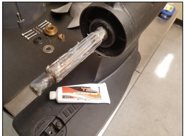
Img 2b. Inspect the propeller shaft, for corrosion, pitting, and straightness
