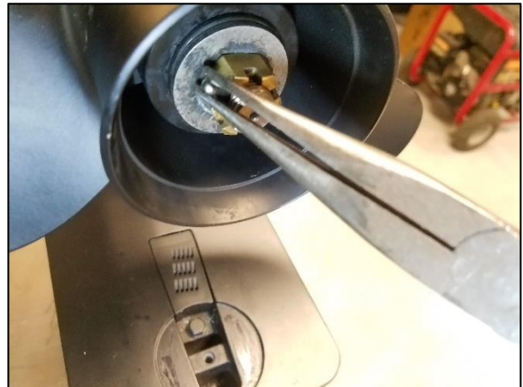
Img 1b. Remove Split Pin with needle nose pliers
