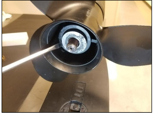
Img 1d. Remove the Stainless-Steel Washer and Stopper from the propeller shaft
