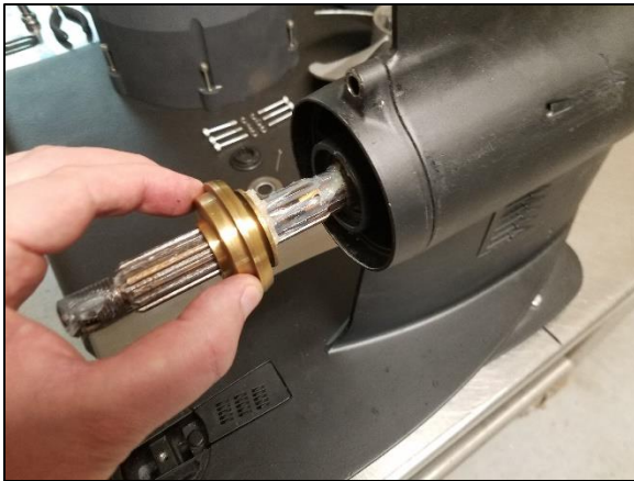
Img 3a. Install the Thrust Washer onto the propeller shaft
