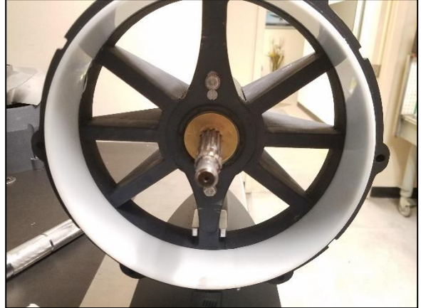
Img 4a2. Brass Impeller Space in place flush with Stator surface.
