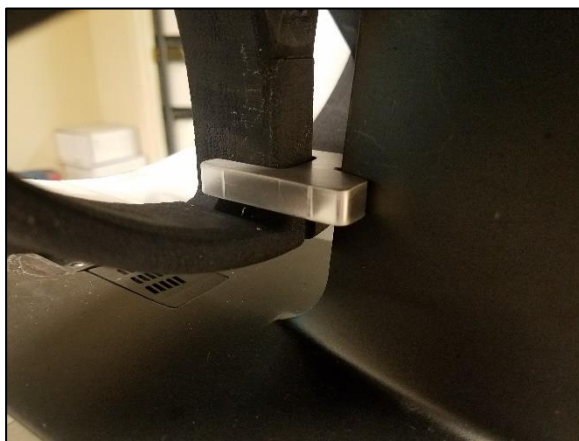
Img 3c. Insert the V-Block between the upper exhaust arm of the Stator and the Lower Unit
