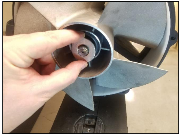
Img 5b. Install the SS Washer and Castle Nut.
