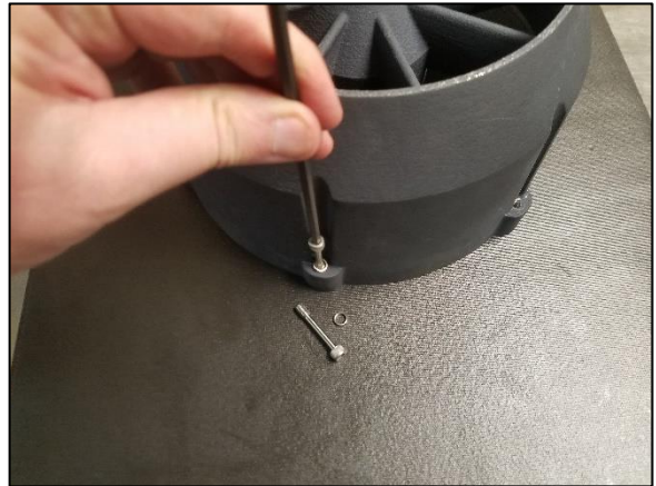
Img 6b. Insert all six (6) of the Captive Screws with High Collar Lock Washers into their
