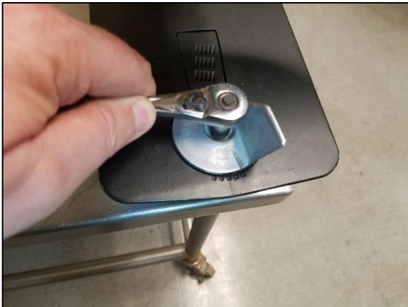
Img 1a. Remove Zinc Anode with 10 mm Socket
