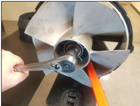
Img 5c. With a 22 mm socket tighten the Castle Nut on the Propeller Shaft
