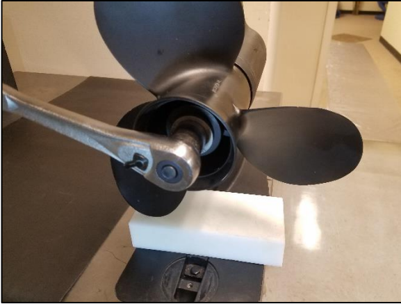
Img 1c. Remove Split Pin with needle nose pliers
