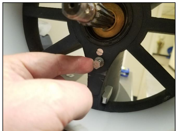
Img 4d. Insert the two (2) Bolts with Nord-lock wedge washer and tighten finger tight
