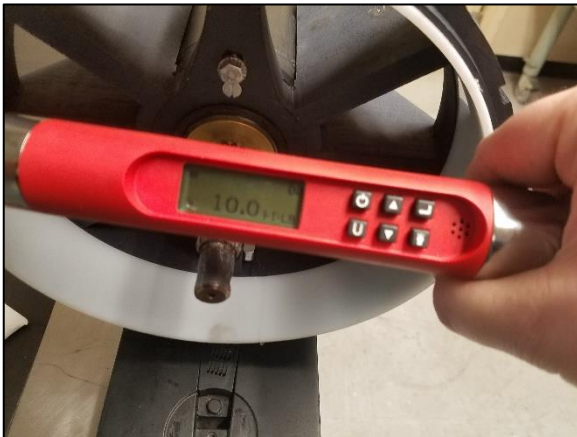
Img 4b. Torque wrench set to 10ft.lbs
