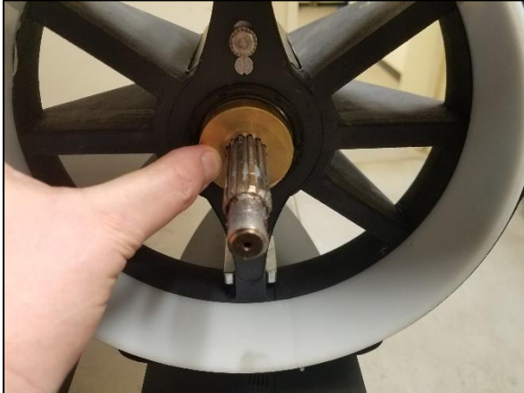
Img 4a1. Apply pressure and push it into place inside the Stator
