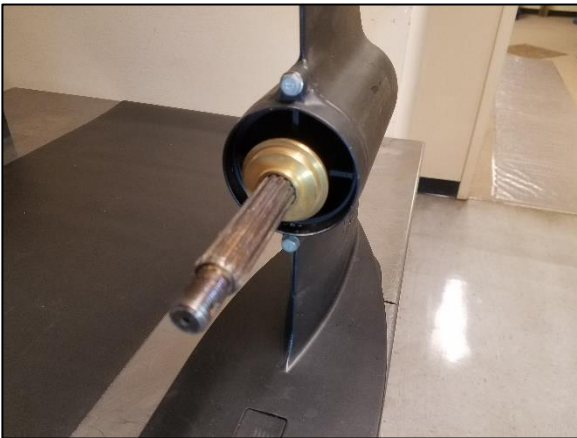
Img 1f. Remove Thrust Washer
