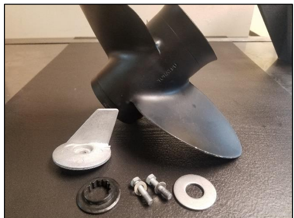
Img 1i. Removed parts required for keep reinstallation of the propeller when required.
