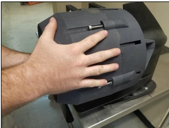
Img 6c. Securely grasp the Nozzle and align with the six mounting holes of the Stator
