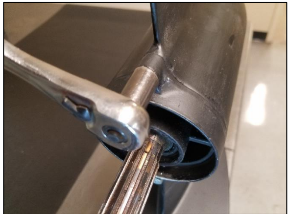
Img 1g. Remove (2) factory 10 mm hex bolts from bearing cap
