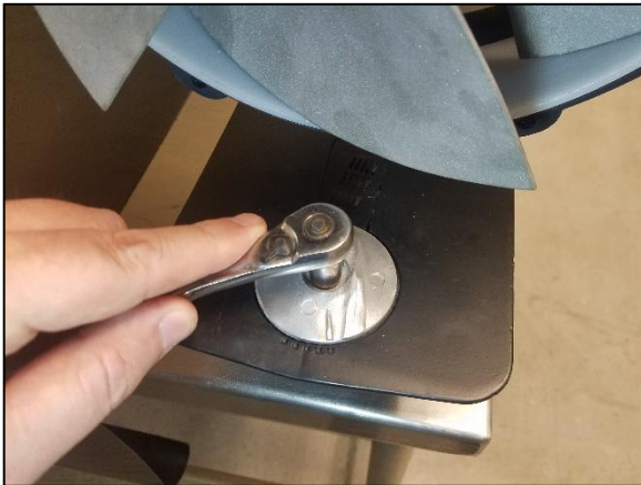
Img 6a. Install the modified Zinc Anode on Anti-Cavitation Plate
